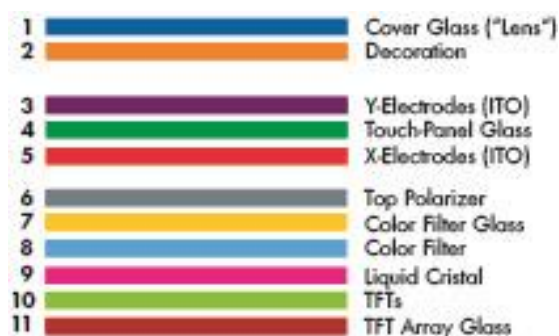
Picture: Construction of a Projection Capacitive Touchscreen
